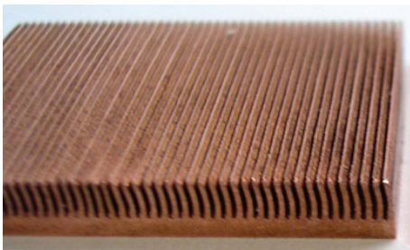
Figure 2. Copper micro-channels used in present work, described as “Fin-H.”
