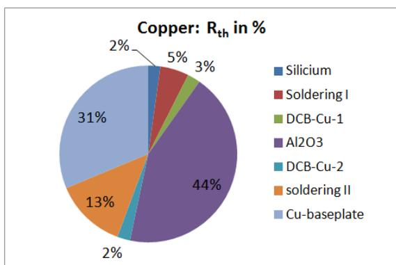
Fig. 4 The relative  $R_{th}$  in % for modules with copper base plates.
