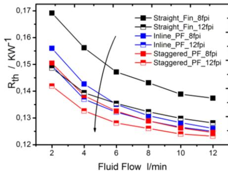
**Fig. 12** Thermal resistance versus the fluid flow (different geometries).
