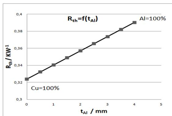
Fig. 7 The absolute  $R_{th}$  is plotted versus the thickness of the aluminium layer. The total thickness  $d_{bp}$  is set to 4 mm
