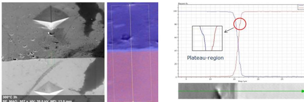
**Fig. 9** The Vickers hardness of the clad material is measured and a line scan with SEM is performed.
