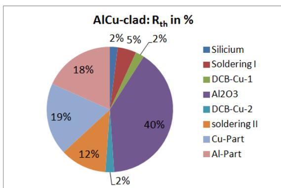
Fig. 6 The relative  $R_{th}$  in % for modules with AlCu-clad base plates (1.5 mm Al, 2.5 mm Cu)
