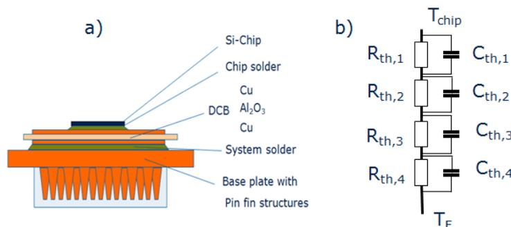
**Fig. 3** a) Simplified cross section of a power module b) The equivalent circuit for the heat transfer, including the thermal resistance and the corresponding capacitances in parallel arrangement
