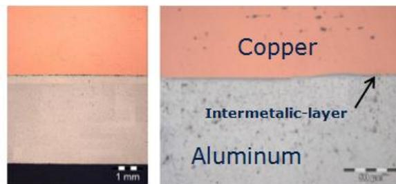
**Fig. 8** A Cross section of the clad material: the different materials and the inter-metallic layer can be recognized clearly.
