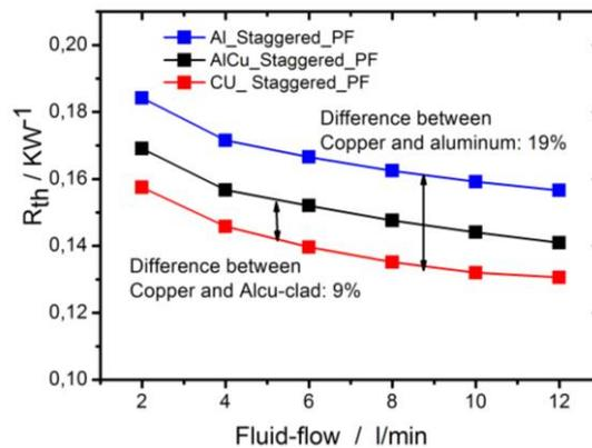
**Fig. 14** The thermal resistance  $R_{th}$  is plotted versus the fluid flow. Different material systems are under consideration
