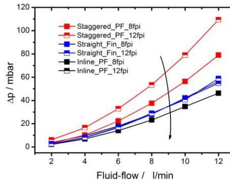
**Fig. 13** Pressure drop versus the fluid flow (different geometries).
