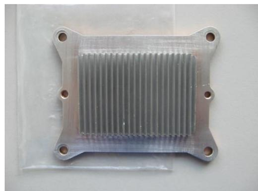
**Fig. 2** Fin structures on the lower side of the base plate for direct cooling.
