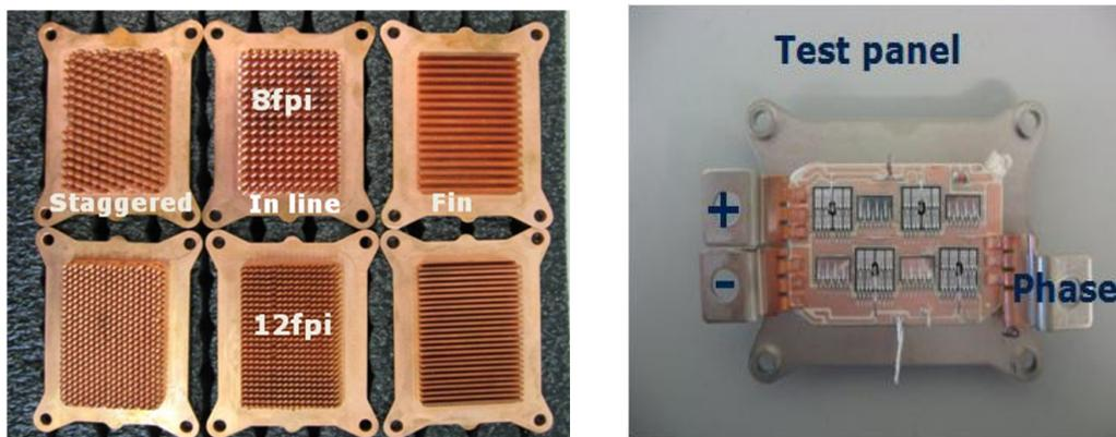
**Fig. 11** Different cooling structures are tested under the same condition. The DUT for  $R_{th}$  measurements is show in right picture
