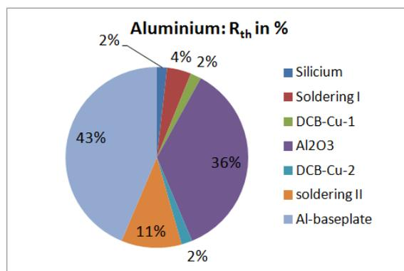
Fig. 5 The relative  $R_{th}$  in % for modules with aluminum base plates.
