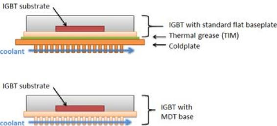
Fig 3. Typical and Integrated Baseplate Cooling Methods
