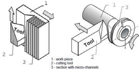
**Fig 5.** Micro Deformation Technology (MDT)
