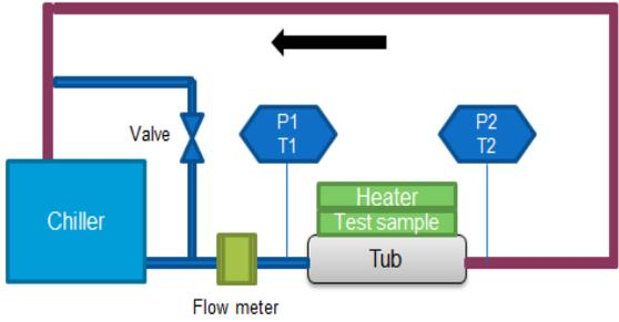
Fig 8. Experimental Test Platform Schematic.
