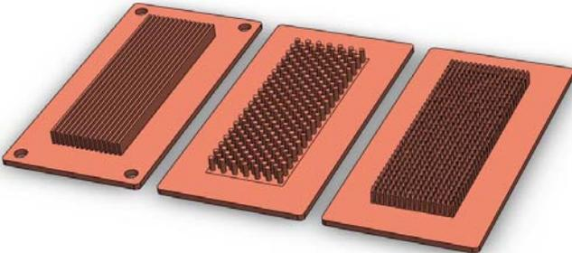
Fig 4. Three geometries tested: straight fin, round staggered pin fin, MDT in-line pin fin.
