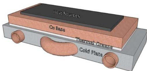
(a) Copper tubes into aluminum slab
