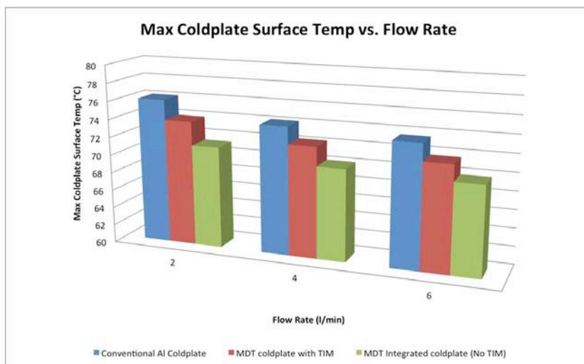
Fig. 7. Max. coldplate surface temperature vs flow rate
