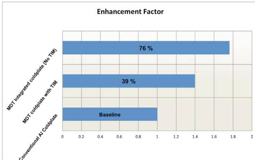
**Fig. 8.** Thermal resistance enhancement factor
