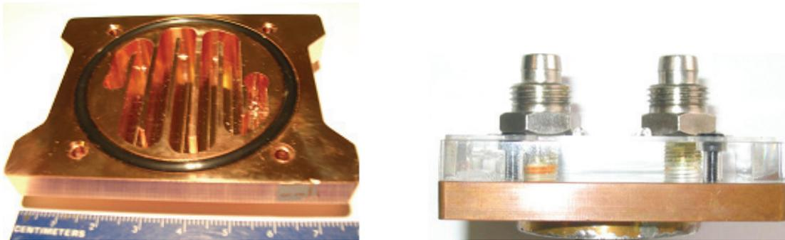
Figure 1 a) Thermaltake “Bigwater” waterblock having one serpentine channel 4.5 mm wide x 10 mm deep, b) Side view with Plexiglas cover and fluid connectors.
