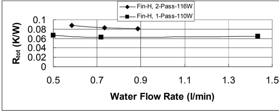
Figure 4.  $R_{tot}$  of 1-pass vs. 2-pass micro-channel coolers.
