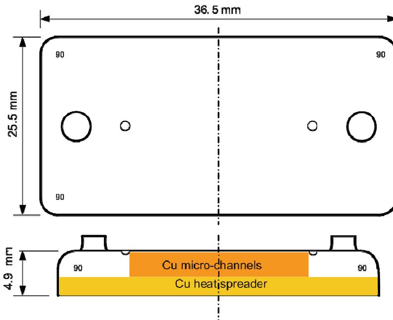
Figure 8. Illustration of fabricated micro-channel cooler.
